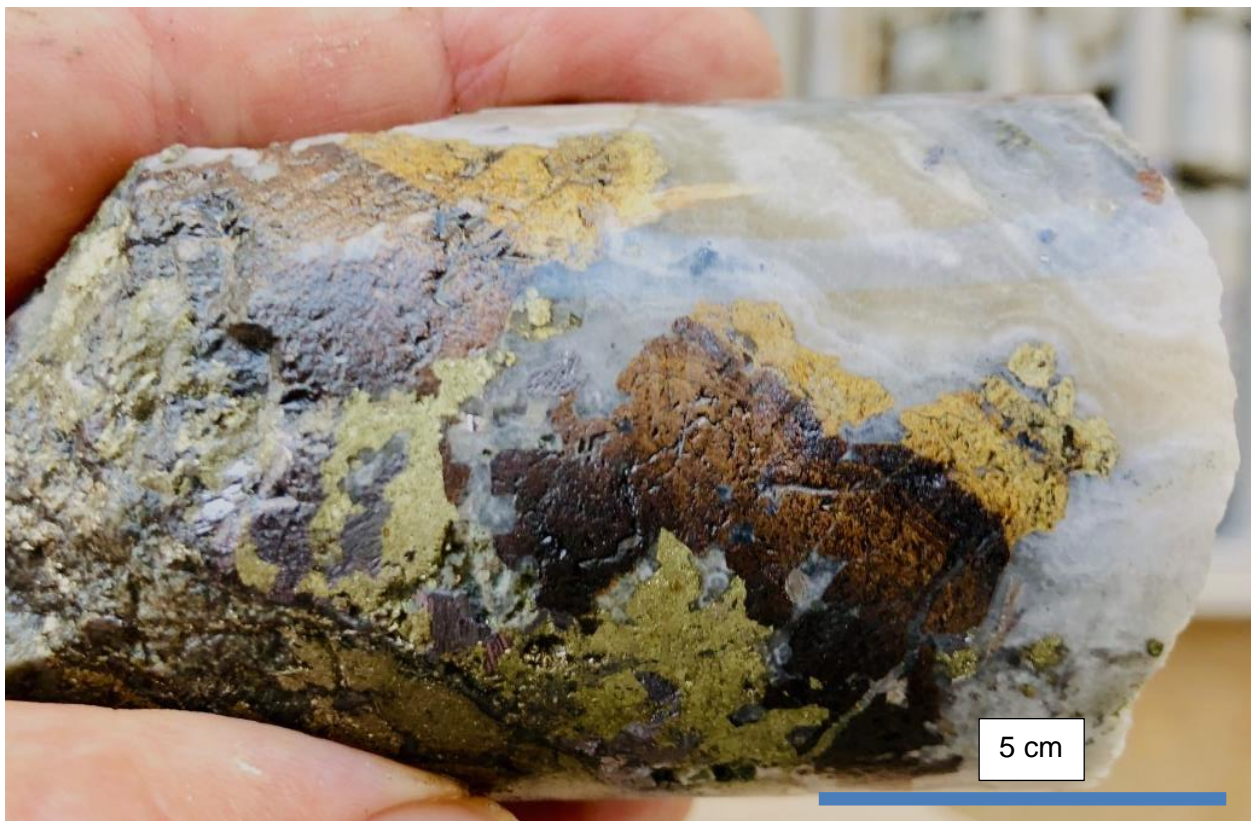
Figure 5. Diamond drill core from 230 metres downhole in RTIPT016. Copper sulphides (chalcopyrite) is yellow coloured at base of core; brown to honey coloured zinc sulphide (sphalerite) in the centre; and colloform to crustiform quartz-chalcedony in upper right.
