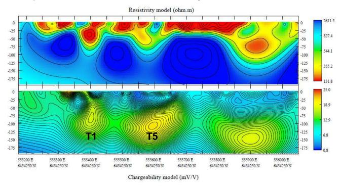
**Figure 3.** Results of ground IP survey along middle traverse on Figure 2 showing the chargeability anomalies that may represent disseminated sulphide at Targets T1 (Red Hill mine) and Target T5).
