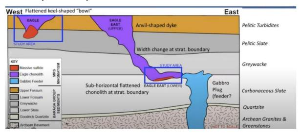
Figure 5: Simplified cross-section through the Eagle and Eagle East deposits.
