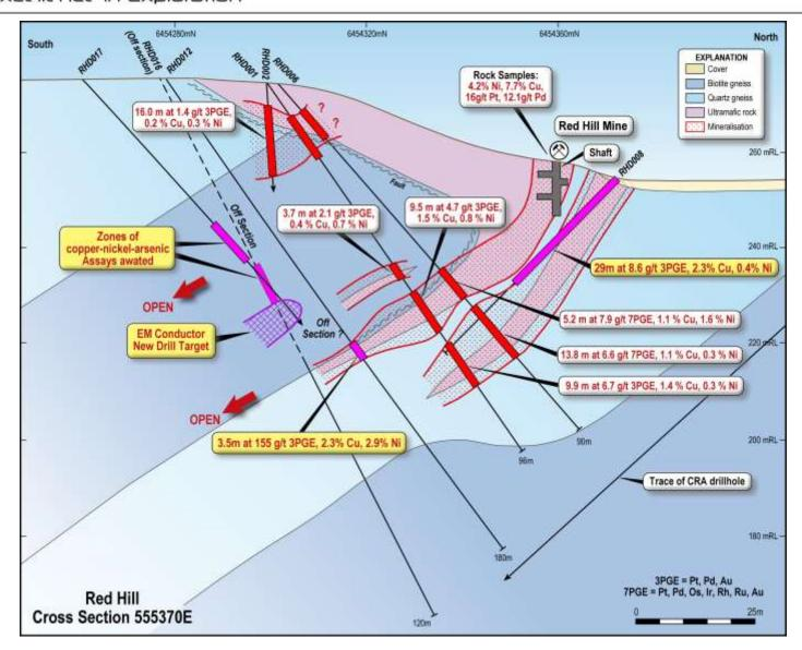
**Figure 1.** Cross section through the Red Hill Prospect.
