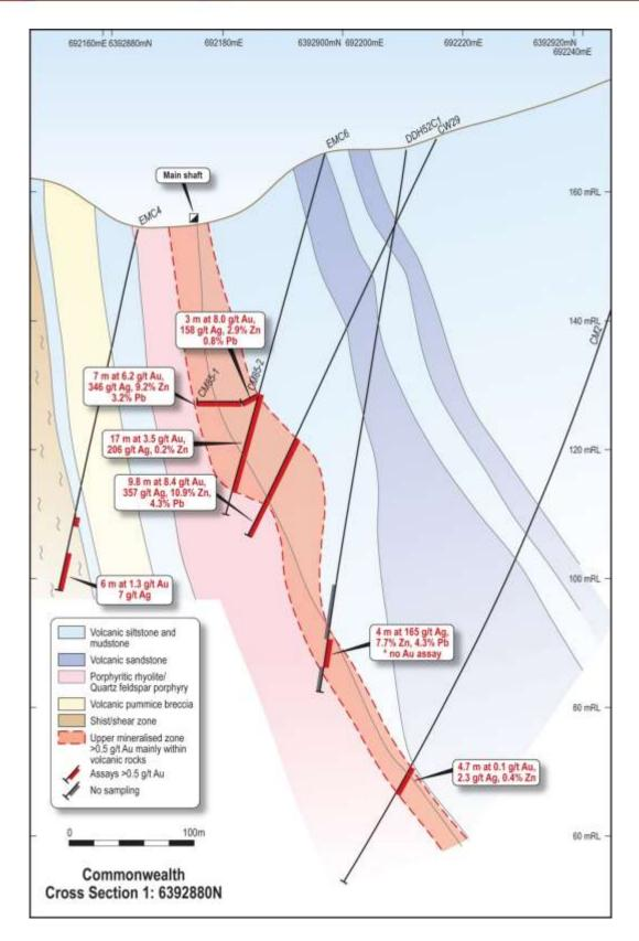
**Figure 6.** Cross section 1 (Figure 5) showing the geology and key drill results beneath the main shaft at Commonwealth.
