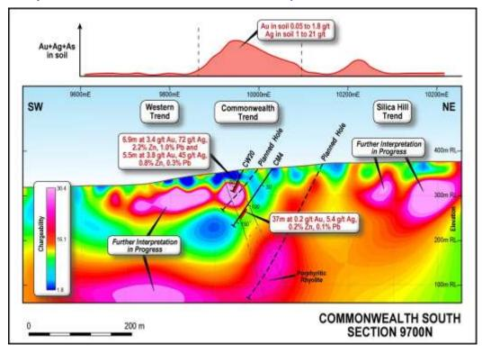
**Figure 2**. Results of an Induced Polarisation Survey over the Commonwealth South Prospect showing the three IP Trends and soil geochemistry responses over the areas. The Western Trend lies beneath alluvial cover (see Figure 1 for location of survey line).
