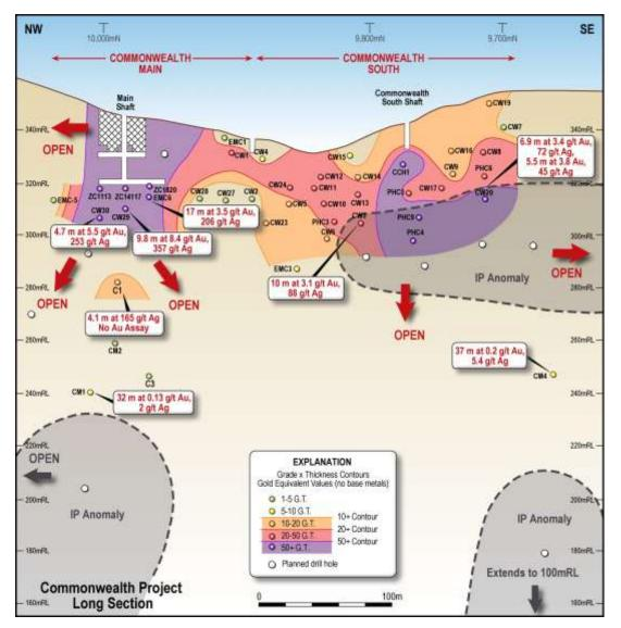
**Figure 3.** Long Section between Main Shaft and Commonwealth South Prospects showing the location of previous drill holes, significant gold and silver mineralisation and the IP anomalies.
