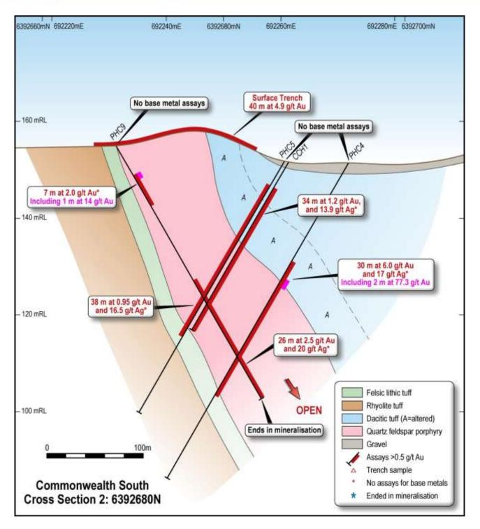
**Figure 7.** Cross Section 2 (Figure 5) showing the geology and key drill results in the centre of the Commonwealth South Prospect.
