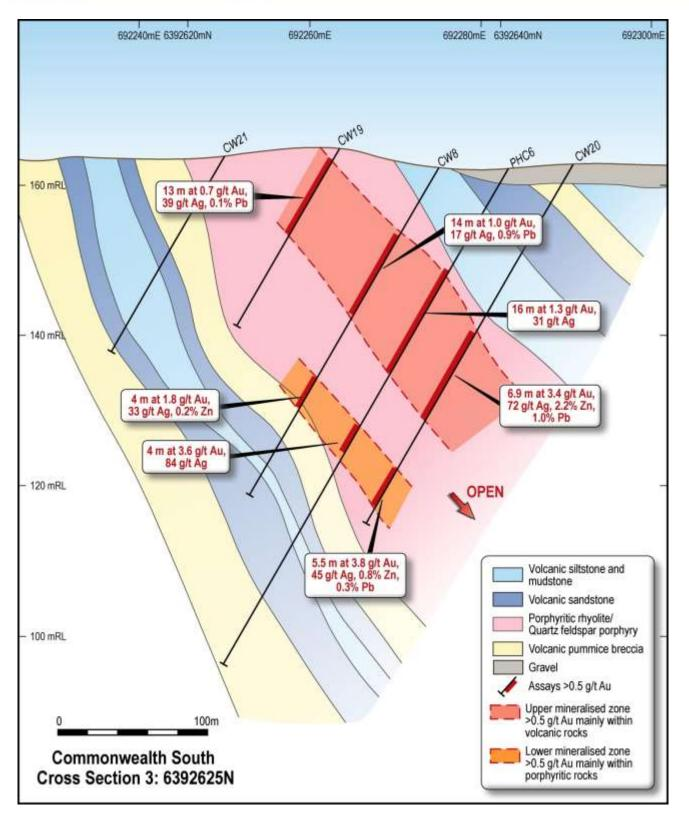
**Figure 8.** Cross Section 3 (Figure 5) showing the geology and key drill results at the southern end of the Commonwealth South Prospect.
