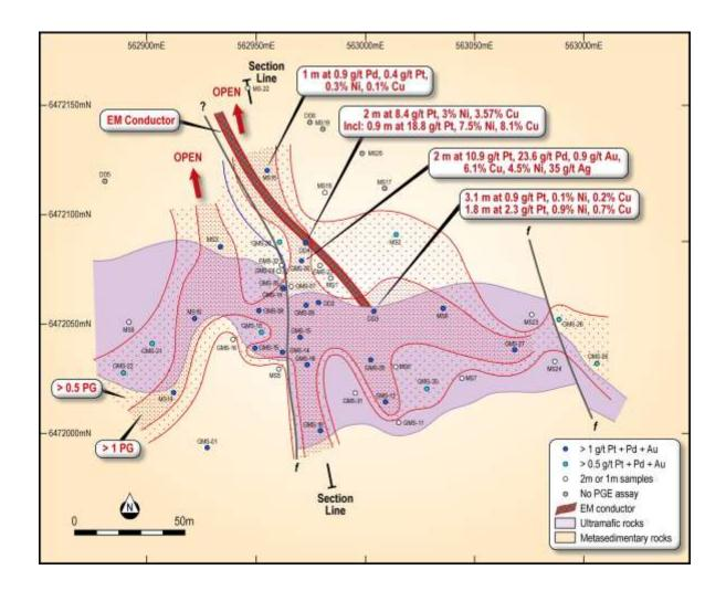
**Figure 1.** Geology, EM anomaly, previous drill holes and contoured data of previous drill assays for platinum, palladium and gold (summed from down hole intervals). The down hole EM survey was completed in Hole GMS-33.
