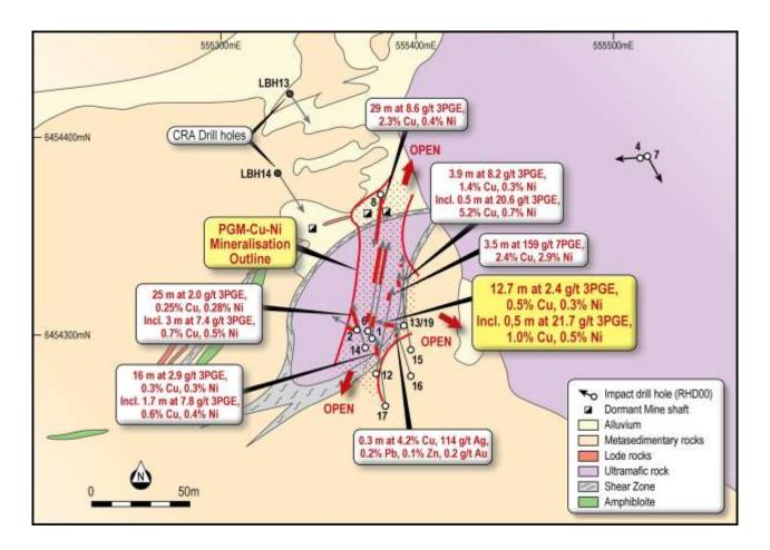
**Figure 2.** Geology and drill hole locations at Red Hill showing the seven significant assays of the current drill programme in holes RHD008, 012, 014, 015, 016, 017 and 019 (in yellow call out box).
