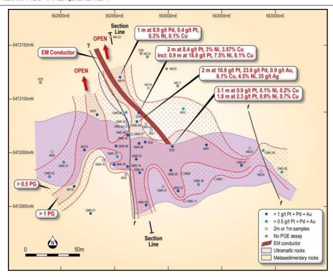
**Figure 3.** Geology, previous drill holes and contoured data of previous drill assays for platinum, palladium and gold (summed from down hole intervals). A strong northerly control in mineralisation is apparent, in contrast to the east-west trend of the host ultramafic. The down hole EM survey was completed in Hole GMS-33.
