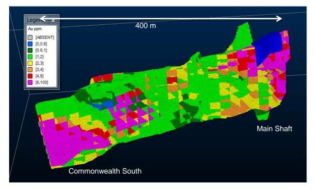
**Figure 2.** Block model of the resource from Commonwealth South (left) to Main Shaft (right). The distribution of the high grade blocks in pink show that the deposit is open along trend and at depth.
