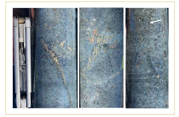
**Figure 1.18.** Photographs of diamond core from selected intervals from 95 m to 98 m down hole in RWIPT016. The photographs show disseminated to blebby to vein hosted sulphide mineralisation comprising pyrite-pyrrhotite-chalcopyrite (copper sulphide) and lesser pentlandite (nickel sulphide). Fine grained disseminated sulphide occurs in many places in this interval (see arrow for example)
