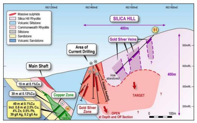
**Figure 11.** Cross section looking north west from Main Shaft to the south and Silica Hill to the north (see Figure 10 for location). Three components to the mineralised system are evident: an upper zone of weakly mineralised gold-silver veins; a middle zone of high grade gold-silver +/- base metal veins and a lower zone of massive sulphide and increasing copper-gold-silver at depth.
