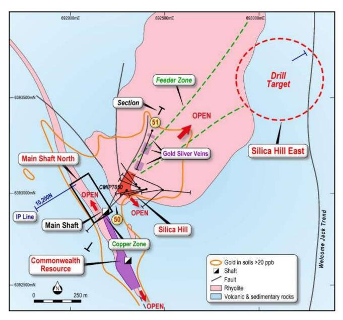
**Figure 10.** Geology of the Silica Hill-Commonwealth area and locations of Holes CMIPT50 and 51. Note that the low grade gold-silver veins in Hole 51, drilled from north east to south west, overlies an interpreted north east trending feeder zone. Hole 50 tested a conductor below Main Shaft and intersected a broad zone of copper sulphide mineralisation.
