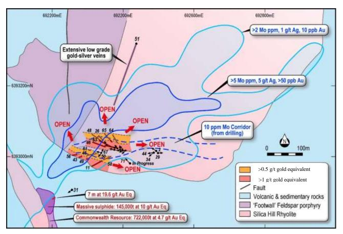
**Figure 8.** Overview of the Silica Hill Prospect showing drill hole locations and east-west trending gold-rich zones within a north east trending corridor defined by a gold-silver-molybdenum-in-soil anomaly. Note that the drilling has only tested the near surface portion of 10% of the target area.
