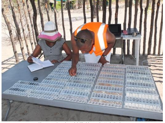
Figure 12. Logging of drill chips at the Xade Project.
