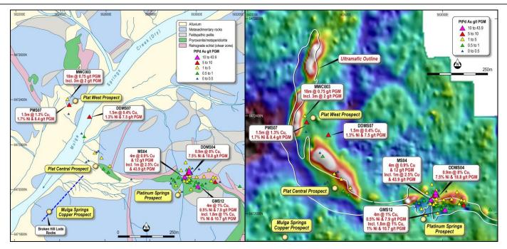
Figure 3 and 4. Surface geology (left) and image of magnetic data (right) of the Platinum Springs area showing key prospects and previous drill results.
