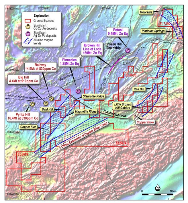
**Figure 1.** Location of Impact's tenements in the Broken Hill area and key prospects for nickel-copper-PGM mineralisation. Platinum Springs, Red Hill and Little Broken Hill Gabbro are in the NE of the map.
