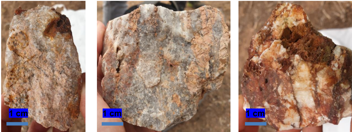
Figure 4. Gradation of veins from K-feldspar dominant (left photo) to quartz-dominant (right photo) with increasing boxwork gossan (dark brown colour) from weathered sulphides.
