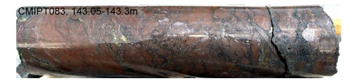
Figure 12. Second massive sulphide unit in Hole CMIPT083: massive and brecciated massive sphalerite (red-brown) with lesser galena. Up to 3% chalcopyrite (yellow) is present in places.
