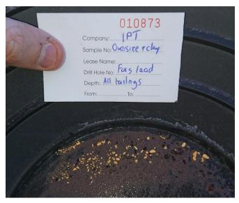
**Figure 5.** Panned concentrate from the re-processing of the first 6 samples which contained sticky clay (Sample 10873 Table 1). Back calculated to the original sample weights this is about 10 parts per billion and attests to the efficiency of the processing method. It is likely that a larger trommel would have captured much of this gold in one phase of processing.
