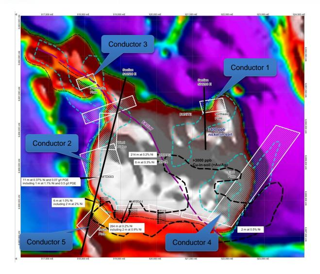
**Figure 4.** Image of the Total Magnetic Intensity from airborne magnetic data over the Mulga Tank Dunite (white outline) showing:
