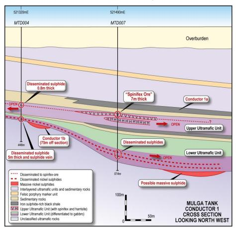
**Figure 1.** Interpreted cross section looking north west, Conductor 1.
