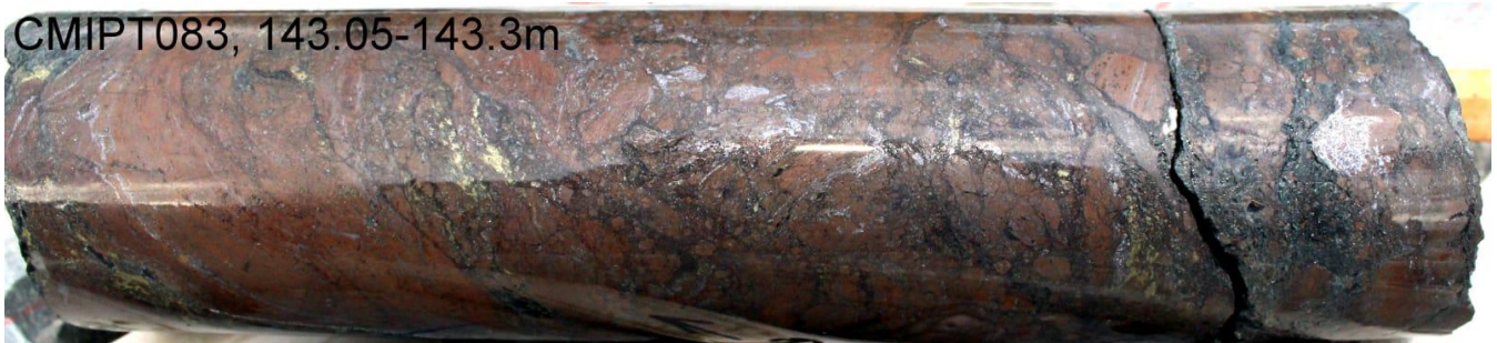
Figure 5. Second massive sulphide unit in Hole CMIPT083: massive and brecciated massive sphalerite (red-brown) with lesser galena. Up to 3% chalcopyrite (yellow) is present in places 2 .
