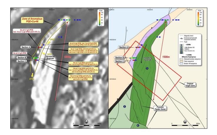
**Figures 4 and 5.** Assay results plotted over airborne magnetic data (left) and an interpretation of the geology from the magnetic data (right). Note the increase in mineralisation to the south and into a target area containing interpreted feeder zones (ASX Release 9<sup>th</sup> July 2020 and 17<sup>th</sup> December 2020). Holes with assays awaited are evident.
