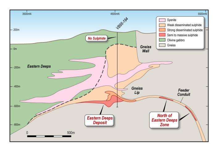
**Figure 9.** Cross-section through the Eastern Deeps deposit at Voiseys Bay. Note the feeder zone to the main intrusion and the large halo of disseminated sulphide mineralisation adjacent to the feeder. The massive sulphide body is some 600 metres deep and there is no surface expression of mineralisation.
