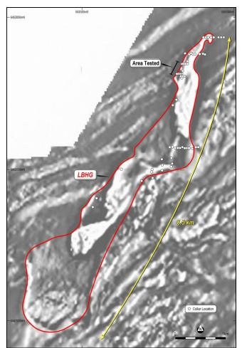
Figure 1. First vertical derivative image of airborne magnetic data over the Little Broken Hill Gabbro showing Impact's drill collars and the area of the basal ultramafic unit tested to date. Drill collars for all of Impact's drill holes completed as part of the reconnaissance programme are shown.
