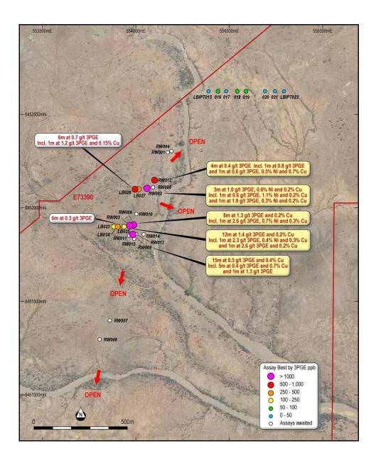
**Figure 2.** Location of Impact's 28 drill holes at Rockwell with best down hole assay result for 3PGE for the 18 drill holes for which assays have been returned from the laboratory.
