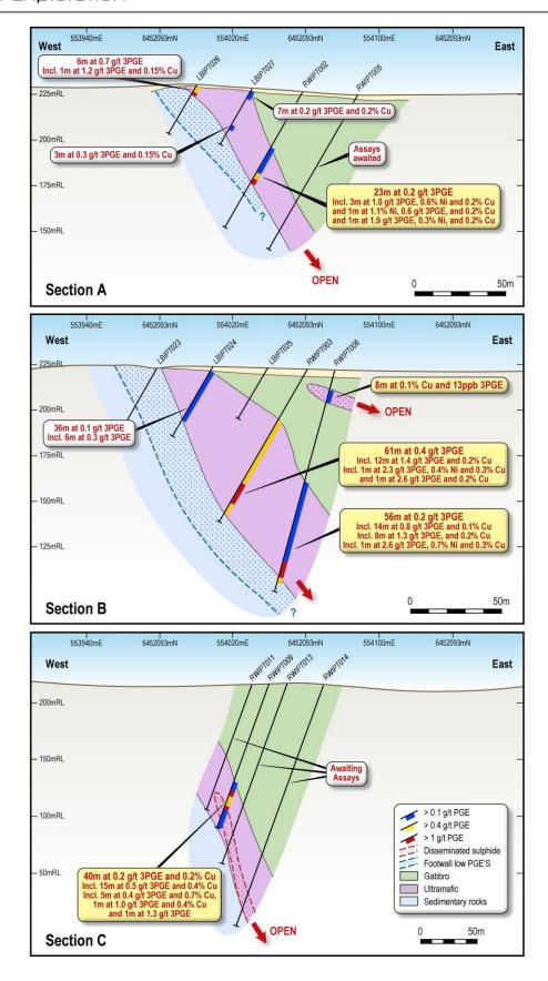
**Figure 3.** Cross-sections through the Rockwell Prospect. Note the increasing sulphide content from north to south. See Figures 3 and 4 for location of cross sections.
