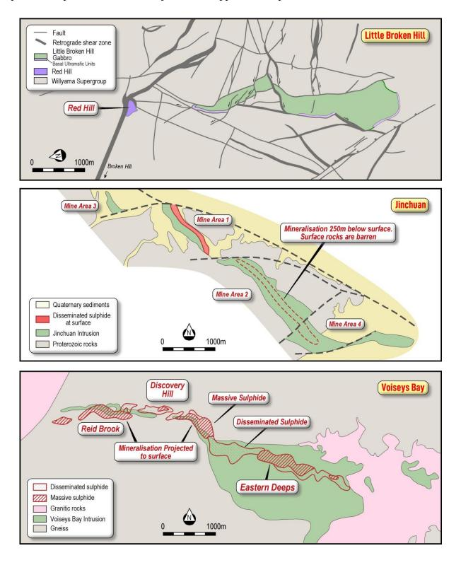
**Figure 11.** Comparison of the Little Broken Hill Gabbro-Red Hill area with Jinchuan and Voiseys Bay. Note the similar scale and also how most of the mineralisation at Jinchuan and Voiseys Bay is at depth.
