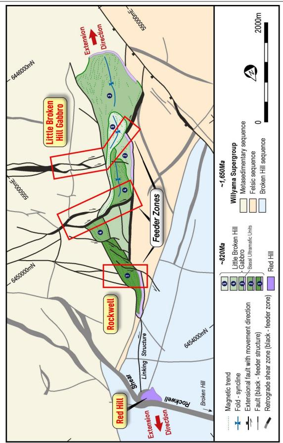
either side of the central of the three possible feeder zones identified. The gabbro has expanded Figure 8. Interpretation of the Little Broken Hill Gabbro. Note the opposite fault slip direction further to the right of this zone (SW) than the left (NE - Rockwell Lobe)
