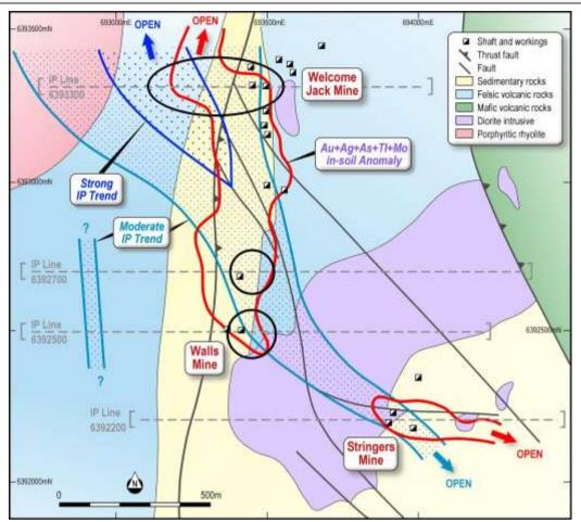
**Figure 2.** Geology and IP and soil geochemistry anomalies at the Welcome Jack Prospect. Three priority drill targets have been identified and are highlighted in the black ellipse and black circles.
