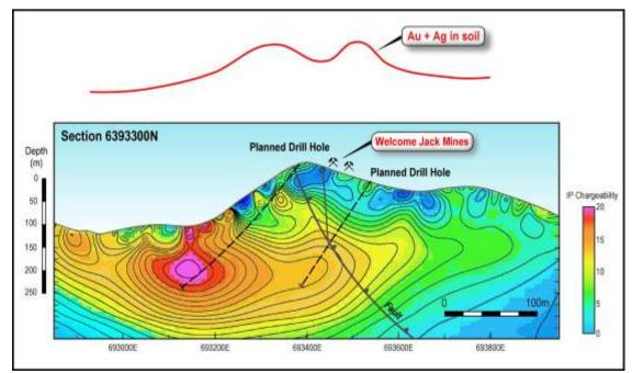
**Figure 3. Welcome Jack Mine:** Cross section of the IP chargeability data on line 6,393,300 mN (Figure 2) with gold and silver-in-soil geochemistry. Two drill holes are planned to test this target area.
