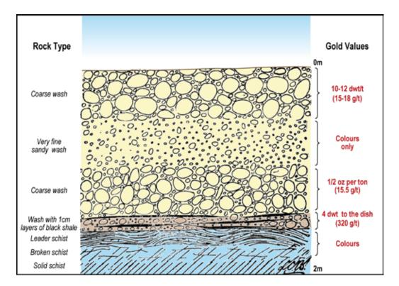
Figure 15. Section from the base of the Bantam shaft at Blackridge (Ball, 1905 GSQ P201)
