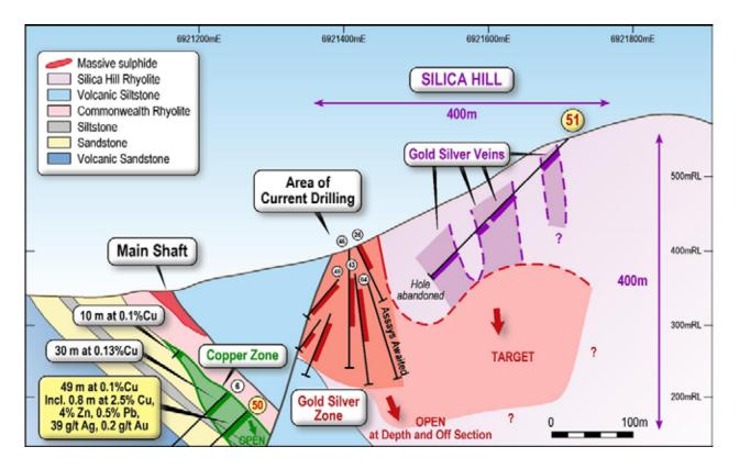
**Figure 3.** Cross section looking northwest from Main Shaft to Silica Hill. Three components to the mineralised system are evident: an upper zone of weakly mineralised gold-silver veins; a middle zone of high grade gold-silver +/- base metal veins; and a lower zone of massive sulphide and increasing copper-gold-silver at depth.
