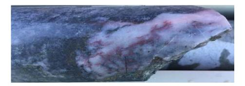
Figure 6. Quartz-ruby silver vein with pyrite and arsenopyrite from 55 m depth in Hole 61.
