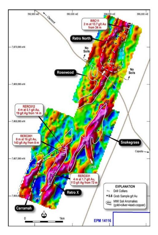
**Figure 12.** Image showing the resisitivity results of the gradient array IP survey at Clermont. The warmer colours are areas of high resisitivity and are likely to be quartz veins. Also shown are the five drill targets and previous relevant drill results.
