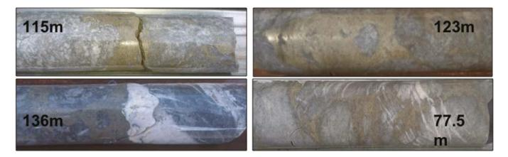
**Figure 7.** Examples of pyrite-arsenopyrite vein styles and orientations from Hole CMIPT64 from down hole depths shown. Similar veins are seen in Holes 65 and 66. All contain silver.
