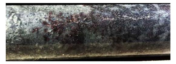
Figure 5. Quartz-pyrite-arsenopyrite-silver vein and stockwork from 77 m depth in Hole 63.
