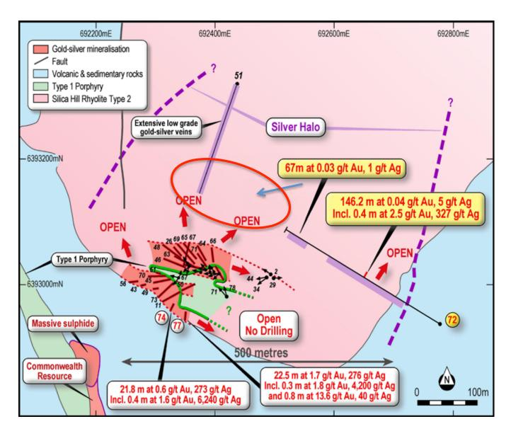
**Figure 8.** Silica Hill Prospect: Geology, drill hole locations and recent significant results. The mineralisation is open and large areas remain to be drill tested.
