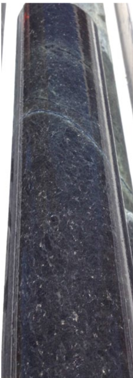
Figure 13a MTD011. Disseminated nickel sulphides in adcumulate dunite interpreted to be of magmatic origin.
