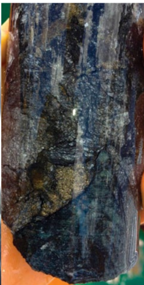
Figure 13b MTD011. Clasts of massive nickel sulphide (with copper sulphide) in breccia zone in dunite. The clast may be remobilised from a nearby body of massive sulphide.
