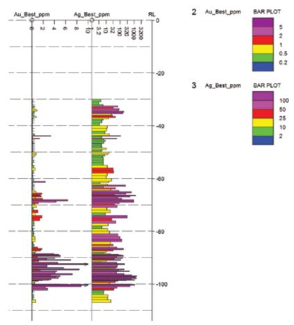
Figure 6. Detail of gold and silver assays for Hole CMIPT046. Note that the gold grades have been cut off at 10 g/t, and silver grades are at log scale to allow proper visualisation of the grades of up to 10 g/t Au and 1,490 g/t Ag.
