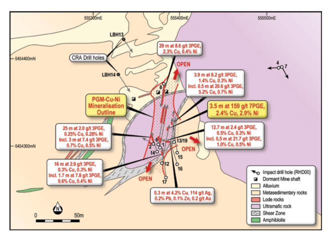
Figure 11. Geology and drill hole locations at Red Hill showing seven significant assays of the 2016 drill programme in holes RHD008, 012, 014, 015, 016, 017 and 019. The standout intercept in hole 012 is highlighted in yellow.
