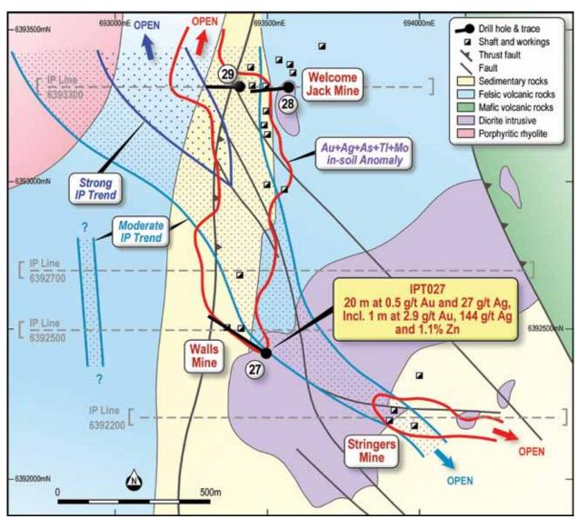
Figure 9: Geology of the Welcome Jack Trend with soil geochemistry, IP anomolies and drill hole locations.
