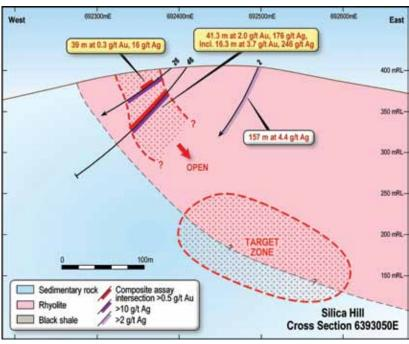
Figure 5. East-West cross section showing results for Holes CMIPT026 and 046.
