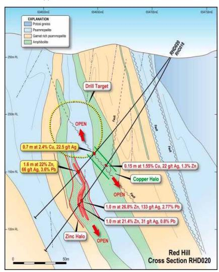
Figure 17. North-South Cross Section for Holes RHD020 and RHD018 looking west.
