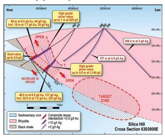
Figure 7. East-West cross section showing results for Holes CMIPT026 and 046.
