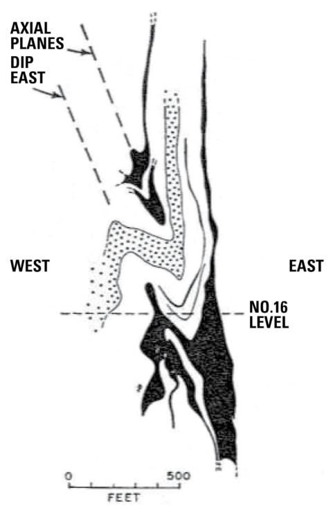
Figure 18. Cross-section through the Broken Hill Mine showing the relationship between fold hinges and thick ore positions (black areas).
