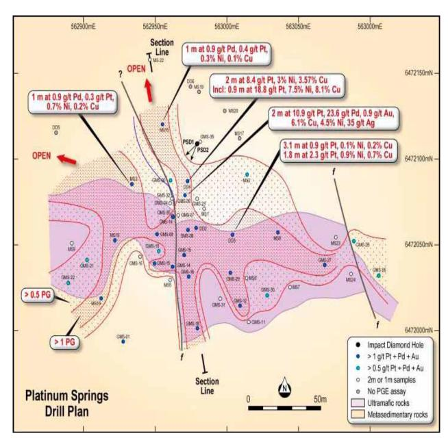
Figure 13. Geology and location of PSD01 and PSD02, previous drill holes and contoured data of previous drill assays for platinum, palladium and gold (summed from down hole intervals).
