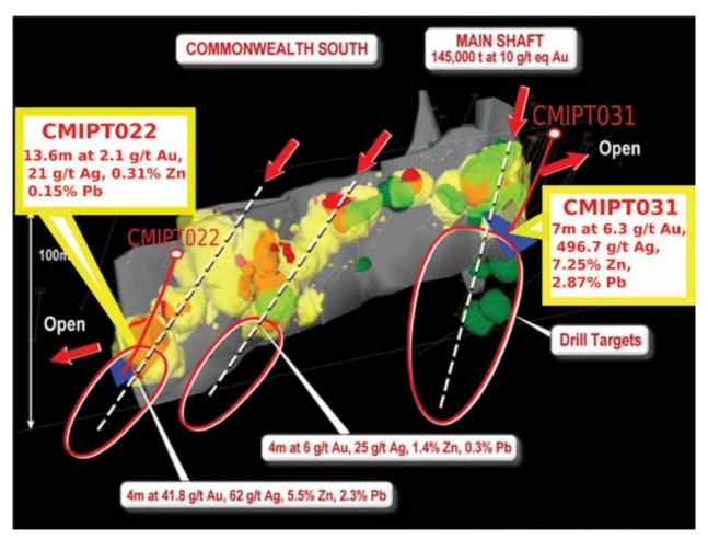
Figure 3. 3D view looking to the north west of the Commonwealth resource (grey outline) and showing: grade shells for gold (yellow = 1g/t, red/orange = 2 g/t) and copper (green = 500 ppm copper) from drill assay data; interpreted EM conductors (blue rectangles) and interpreted ore shoots (dashed lines). Recent drill holes CMIPT022 and CMIPT031 indicate mineralisation is open down plunge in at least 2 areas
